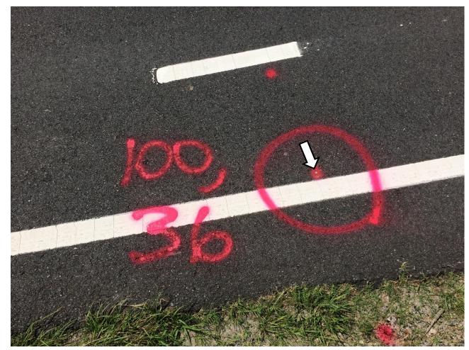
A. Photo showing PK nail (at arrow) set at one of four corners of GPR grid.
